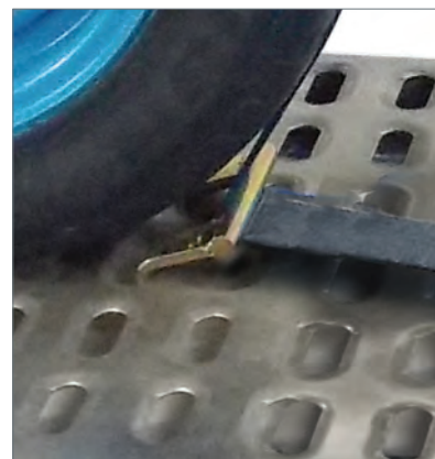
Trailer deck holes running horizontally across the deck.
